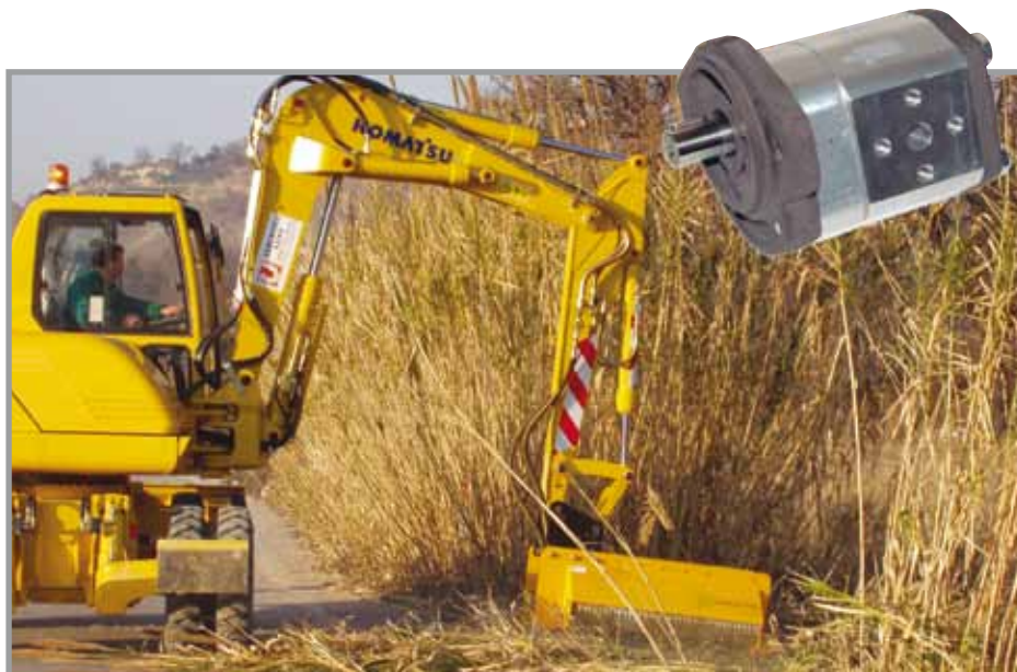
A typical gear motor application: bush cutter with T-system gear motor
