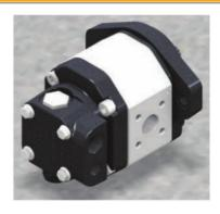
The V30E-270 has been designed for an operating pressure of up to 5,075psi (350 bar), with a peak pressure of 6,000psi (420 bar). The output volume is up to a maximum of 124gal/min (470 litres) at 1,750rpm, with a geometric displacement of 270cc/rev.
