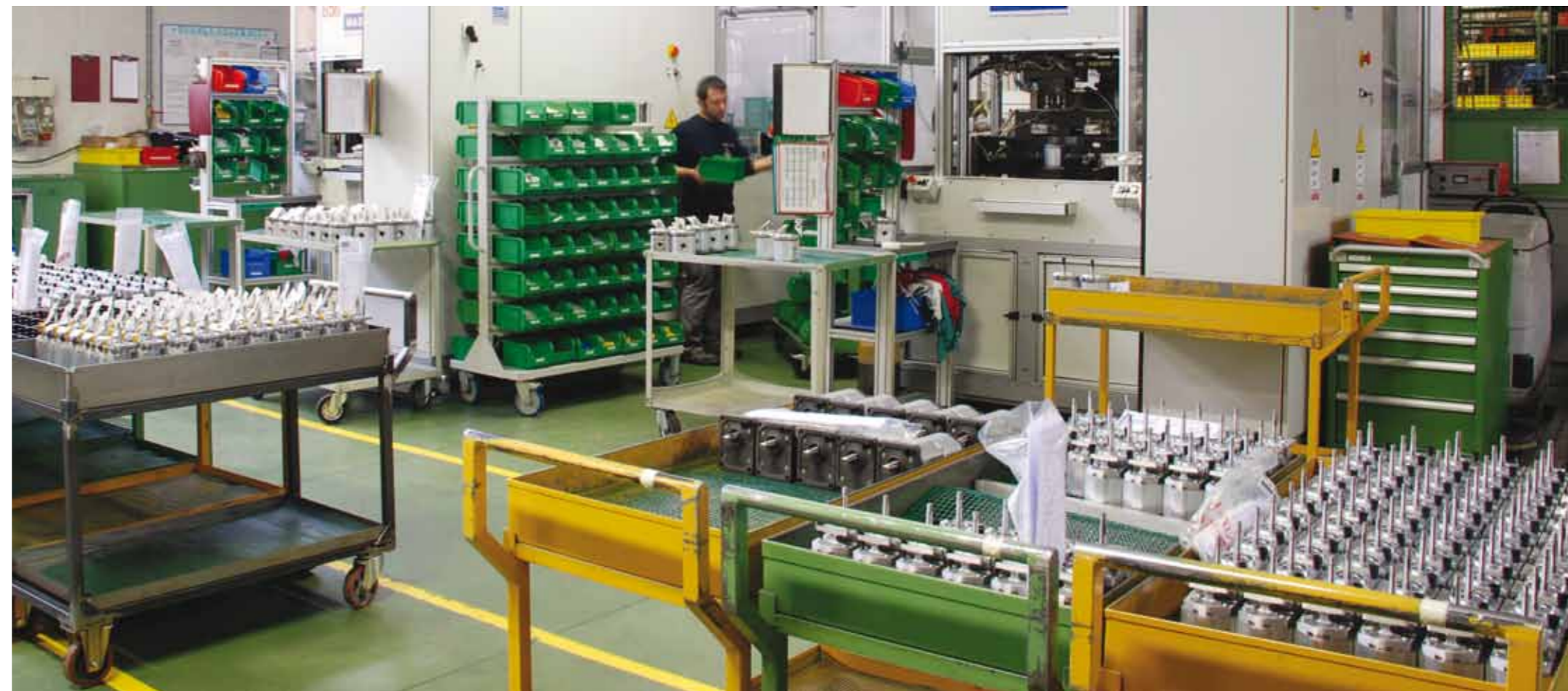
FIGURE 3: Marzocchi Pompe factory, the running-in department
