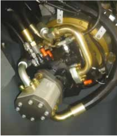
FIGURE 1: Liebherr application of Marzocchi GHP3AD-66-S1 gear pump
