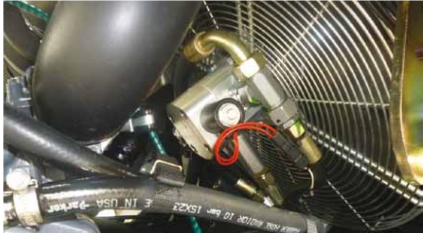
FIGURE 2: Liebherr application of Marzocchi ALM2BK1-D-12 gear motor with electro proportional valve and gauge port
