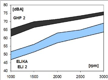
Noise pump comparison [dBA] Marzocchi GHP2 — ELIKA ELI 2, same displacement 17.8 cm³/rev, pressure from 10 to 250 bar.
