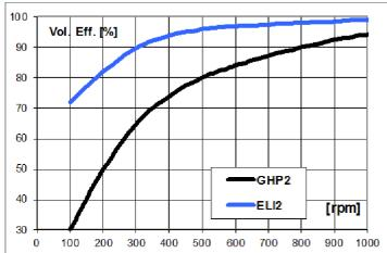
Comparison of volumetric efficiency at low rotation speed: Marzocchi
