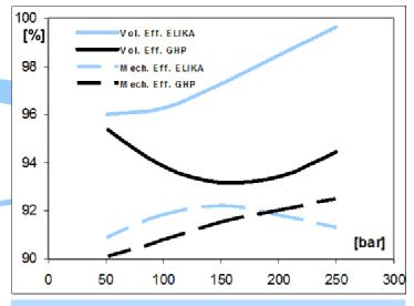
Efficiency pump comparison [%] Marzocchi GHP2 — ELIKA ELI 2, same displacement 17.8 cm $^3$ /rev, rotation speed 1500 rpm.
