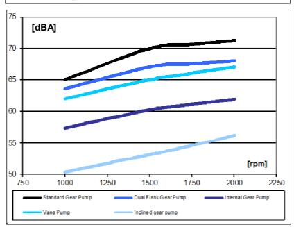
The low pulsation reduces the induced vibration in the machines. The lower frequency of the ELIKA pump produces a more pleasant sound. Pressure pulsation comparison between: standard external gear pump, dual flank gear pump, ELIKA pump, pressure 200 bar, rotation speed 1500 rpm.
